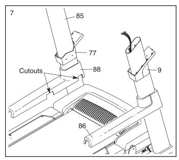
8. Remove the band securing the Upright Wire Harness (73) to the right Upright (85). Have a second person hold the console assembly near the right Upright.
